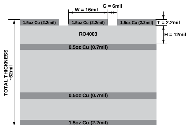
Figure 27. Evaluation Board Stackup, Cross Sectional View
