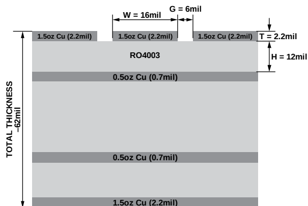
Figure 37. Evaluation Board Stackup
