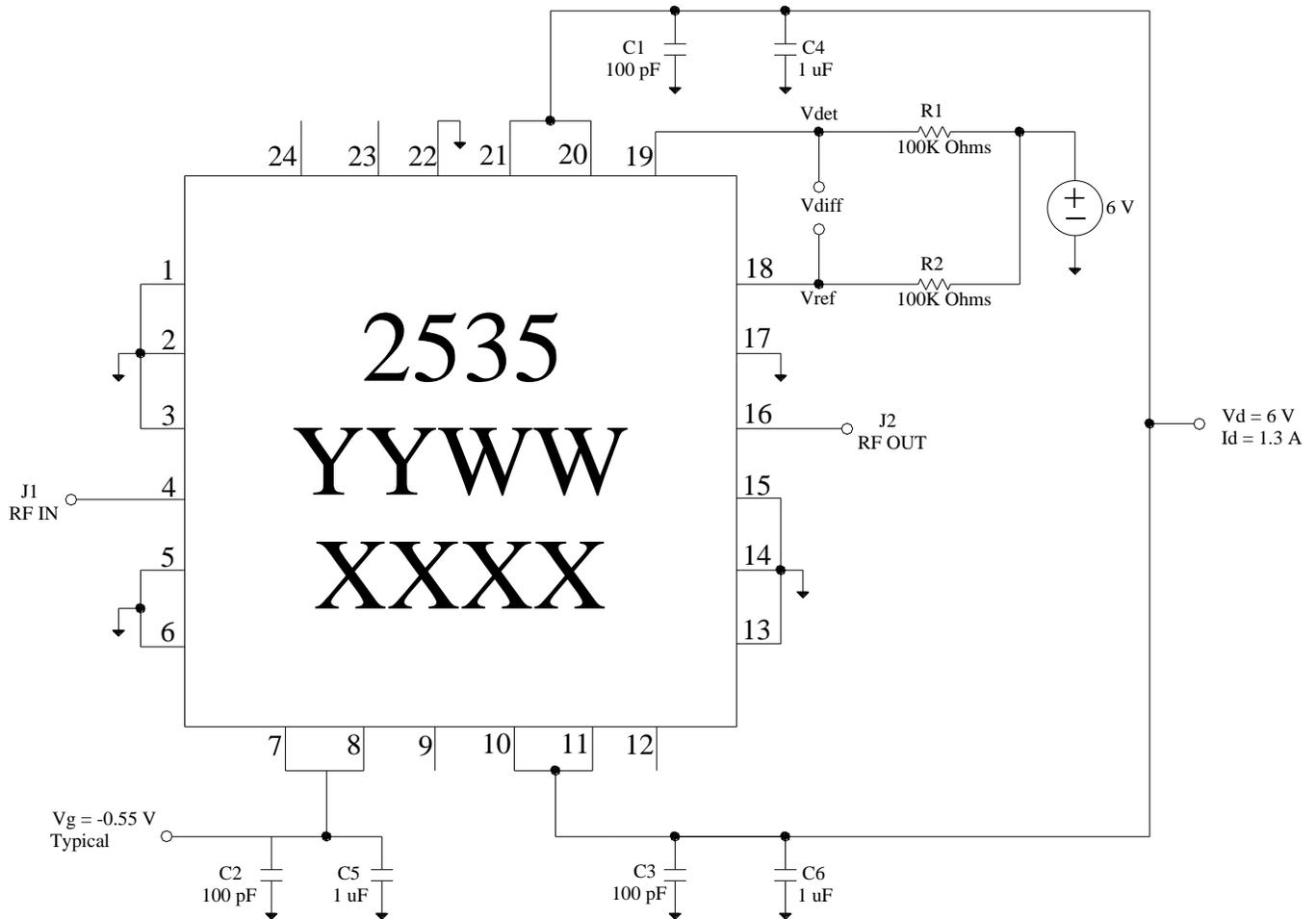
Vg can be biased from either side (pins 7 and 8 or pins 23 and 24), and the non-biased side can be left open.
