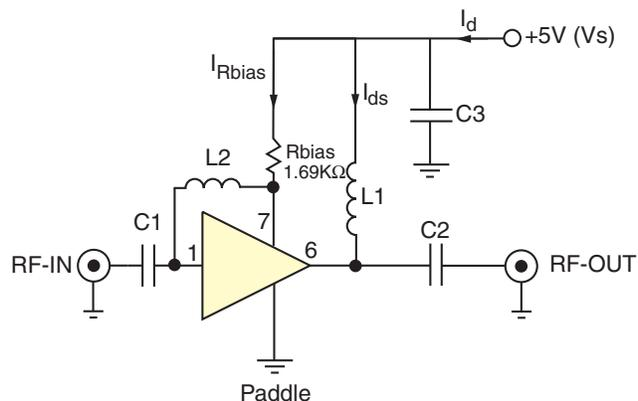
**Fig 3.** Recommended Application Circuit
