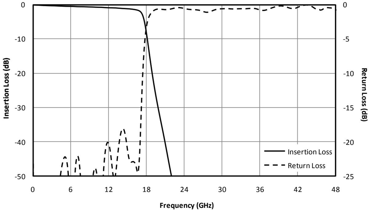
Fig. 1. Magnitude response for a typical FLP-1740.
