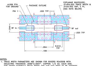
ITRACE WIDTH PARAMETERS ARE SHOWN FOR ROGERS R04350B WITH DIELECTRIC THICKNESS .0066°±.0007". COPPER: 1/2 02. EACH SIDE. FOR OTHER MATERIALS TRACE WIDTH AND GAP MAY NEED TO BE MODIFIED.
