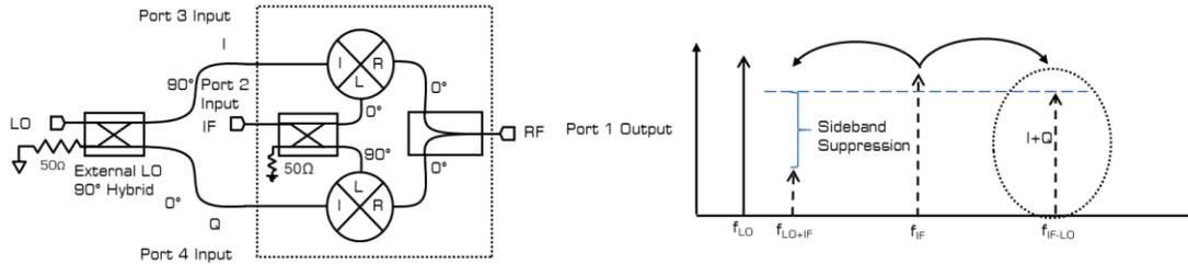
A band shifter is an unusual application for a mixer. Band shifters take an IF signal and shift it to a different band, generally to either avoid interference or for rebroadcast at a different frequency. For cases in which the desired band shift cannot be employed by using a standard up or down conversion scheme, an exotic input scheme is required.
