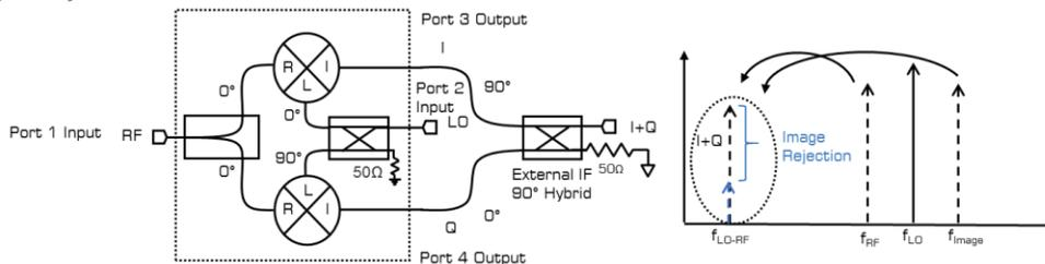
An image reject mixer is a mixer which rejects the down converted image frequency from the IF output. Image reject mixers are constructed using an external quadrature hybrid attached to the I and Q (i.e., IF) output ports of an IQ mixer. Using the external IF quadrature hybrid, one can select whether the upper sideband or lower sideband signal is suppressed with respect to the LO signal.
