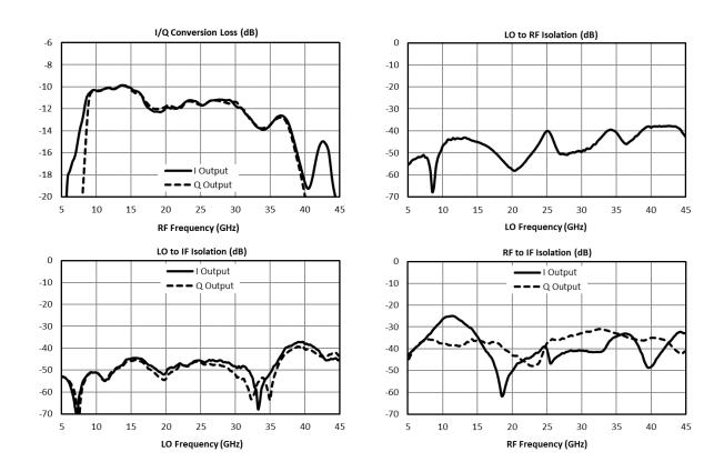
$<sup>^{\</sup>rm 6}$  I+Q measurements taken with an external quadrature hybrid attached to the I and Q ports of the mixer. Orientation depends on up conversion or down conversion measurement.
