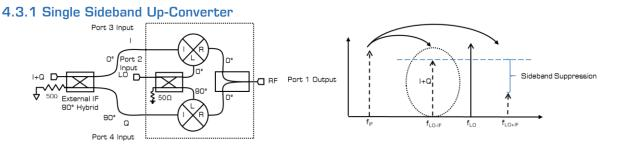
A single sideband mixer is a mixer which suppress the up converted image frequency from the RF output. Single sideband mixers are constructed using an external quadrature hybrid attached to the I and Q (i.e., IF) input ports. Using an external IF quadrature hybrid, one can select whether the upper sideband of the lower sideband signal is suppressed with respect to the LO signal.
