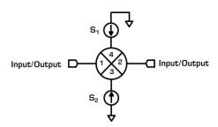
A vector modulator is a device that can modulate an input signal's amplitude and phase. Similar to using a double balanced mixer as a phase modulator or phase shifter, an IQ mixer can be used as a vector modulator. An IQ mixer can be used as a vector modulator by inputting DC current into both the I and  $\mathbb Q$  ports.
