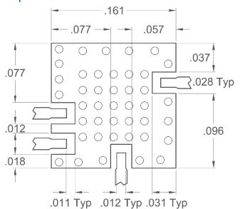
QFN-Package Surface-Mount Landing Pattern
