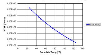
MTTF is calculated from accelerated life-time data of single devices and assumes an isothermal back-plate.
