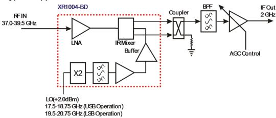
M/A-OOM Tech MMIC-based 30.0-46.0 GHz Receiver Block Diagram (Changing LO and IF frequencies as required allows design to operate as high as 46 GHz)
