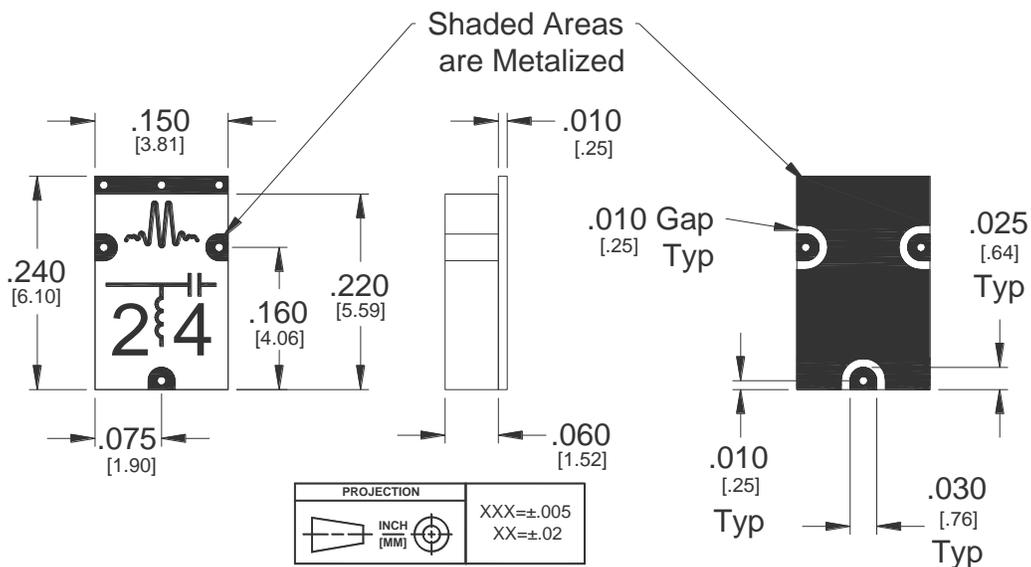
Substrate material is 10-mil thick Rogers 5880 or Taconic TLY-5, ½ Oz Electrodeposited Cu.
